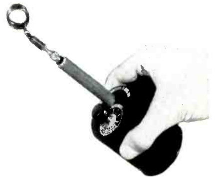
Fig. 2—Actual photo of Probemeter illustrates ease with which it may be applied to circuits being tested. Complete unit is shielded.
